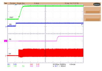
Figure 14. Power Up Sequence and Power Good ( $V_{IN}$  = 3.6 V,  $V_{OUT}$  = 1.8 V,  $I_{OUT}$  = 0 A, L = 1  $\mu$ H,  $C_{OUT}$  = 10  $\mu$ F)
