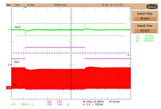
Figure 12. Load Transient Response (V<sub>IN</sub> = 3.6 V, V<sub>OUT</sub> = 1.8 V, I<sub>OUT</sub> = 500 mA to 1500 mA, L = 1  $\mu$ H, C<sub>OUT</sub> = 10  $\mu$ F)
