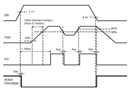
Figure 19. Power Good and Active Discharge Timing Diagram
