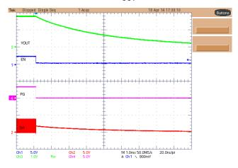
Figure 15. Power Down Sequence and Active Output Discharge (V<sub>IN</sub> = 3.6 V, V<sub>OUT</sub> = 1.8 V, I<sub>OUT</sub> = 0 A, L = 1  $\mu$ H, C<sub>OUT</sub> = 10  $\mu$ F)
