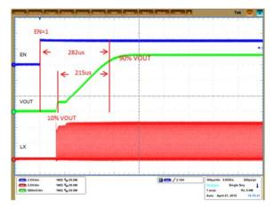
Figure 18. Soft-start Time for NCP6323D ( $V_{IN}$  = 4.2 V,  $V_{OUT}$  = 1.8 V,  $I_{OUT}$  = 0 A, L = 1 µH,C<sub>OUT</sub> = 10 µF)
