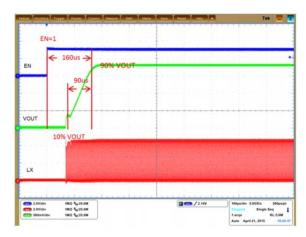
Figure 17. Soft–start Time for NCV6323 ( $V_{IN}$  = 4.2 V,  $V_{OUT}$  = 1.8 V,  $I_{OUT}$  = 0 A, L = 1 µH,C<sub>OUT</sub> = 10 µF)
