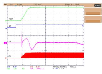
Figure 13. Power Up Sequence and Inrush Current in Input (V<sub>IN</sub> = 3.6 V, V<sub>OUT</sub> = 1.8 V, I<sub>OUT</sub> = 0 A, L = 1  $\mu$ H, C<sub>OUT</sub> = 10  $\mu$ F)
