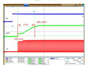
Figure 16. Soft-start Time for NCP6323D ( $V_{IN}$  = 4.2 V,  $V_{OUT}$  = 1.1 V,  $I_{OUT}$  = 0 A, L = 1 µH,C<sub>OUT</sub> = 10 µF)
