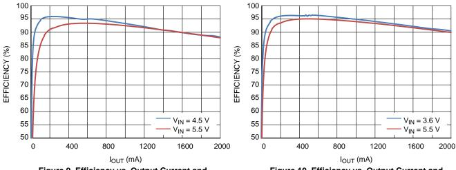
Figure 9. Efficiency vs. Output Current and Input Voltage ( $V_{OUT}$  = 3.3 V,  $T_A$  = 25°C)
